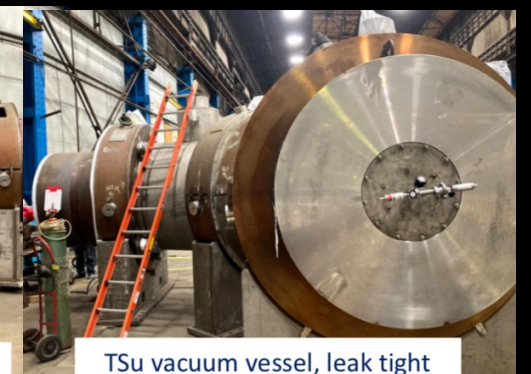
TSu vacuum vessel, leak tight
