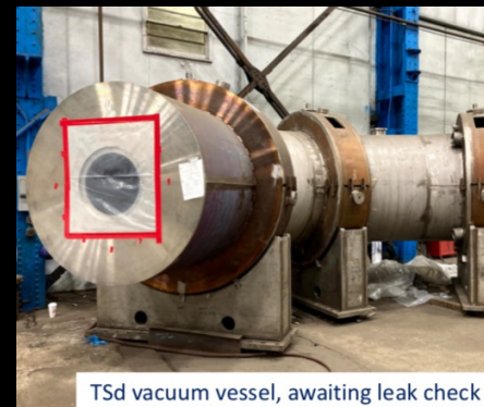
TSd vacuum vessel, awaiting leak check
