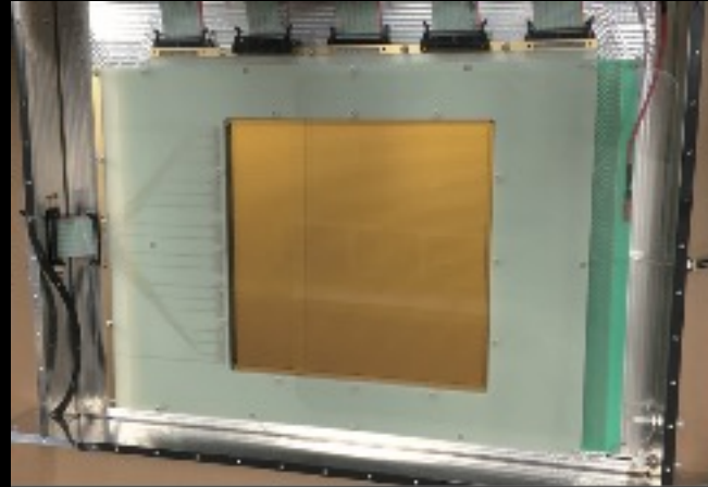
Inside of a multiwire proportional chamber used in the DeeMe experiment.
